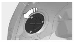
In the wheel house, turn the cover counterclockwise and remove it.
