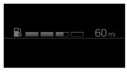
The fill level bars indicate the available fuel supply of the Range Extender when operating readiness and drive readiness are switched on.
