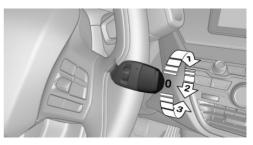
Turn the switch from idle position 0 upward, arrow 1: interval mode. When reverse gear is engaged, the system switches to continuous operation.
