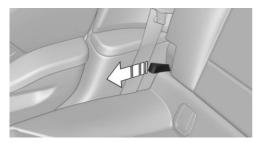
Pull the corresponding loop on the seat backrest forward.
