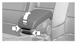
To open, press button, arrow 1. To open, press button, arrow 2.
