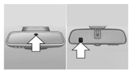
Photocells are used for control:
