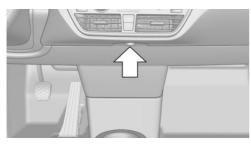
The socket is located underneath the instrument panel. Remove the cover.
