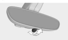
To reduce the blinding effect of the interior rear view mirror, flip the lever forward.
