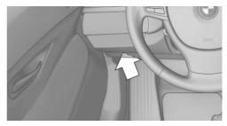
Located on the driver's side is an OBD socket for reading the vehicle data. On vehicles with Range Extender, additional components are checked that are critical for its emissions mix.
