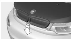
From approx. 16 in/40 cm height allow to fall and press again to lock the hook completely. Make sure you hear the hood engage.
