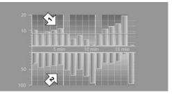
The top bars indicate the average energy consumed while driving time, arrow 1. The lower bars indicate the average energy recovered while driving time, arrow 2.
