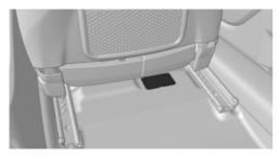
The vehicle identification number can be found under a cover under the front passenger seat.
