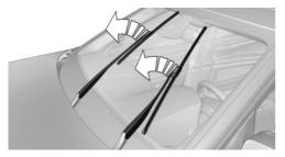
Position the wiper blade in a horizontal position. 4. Remove the wiper blade toward one side.
