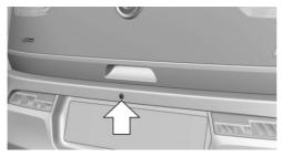
The camera lens is located underneath the tailgate. The image quality may be impaired by dirt. Clean the camera lens, refer to page 203.
