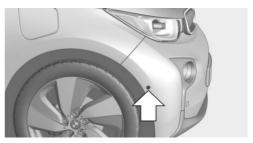
The ultrasound sensors for measuring parking spaces are located on the side of the vehicle.
