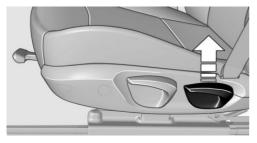
Pull the lever and apply your weight to the backrest or lift it off, as necessary.
