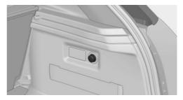
The socket is located on the right side in the trunk. Remove the cover.
