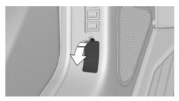
Remove wire cable and pull it back. The hood is unlocked and slightly raised.
