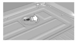
6. Carefully insert the dipstick up to the stop in the measuring tube, and pull it back out.
