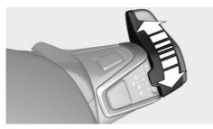
Turn the selector lever in the desired direction.
