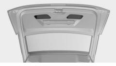
Recessed grips on the inside trim of the tailgate can be used to conveniently pull down the tailgate.
