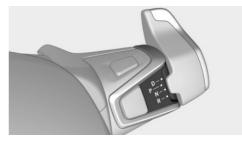
The engaged selector lever position is displayed on the selector lever.
