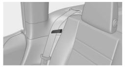
Before folding down the backrest, make sure that the belt is located in the belt buckle.
