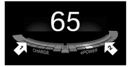
The energy recovery occurs during coasting and braking and is displayed in the performance display by the accelerator pedal indicator.
