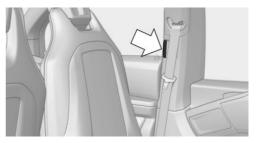
The rear doors can only be opened using the handle on the inside, arrow. The corresponding front door must be opened.
