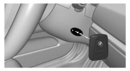
If a respective Check Control message appears, hold the remote control with its back against the marked area on the steering column. The BMW logo on the remote control should be at the same height as the marked area. Press the Start/Stop button within 10 seconds while pressing the brake pedal.
