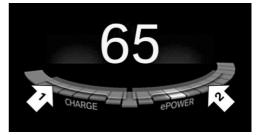
The accelerator pedal indicator in the performance display indicates the current efficiency of the driving style. The efficient range of the performance display is colored blue.
