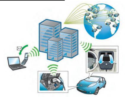
This vehicle incorporates a communication device that is called a TCU (Telematics Communication Unit). The communication connection between this unit and the NISSAN CARWINGS Data Center allows for various services.
