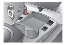
Connect the iPod<sup>®</sup> cable to the USB connector. If the iPod<sup>®</sup> supports charging via USB, the battery of the iPod<sup>®</sup> will be charged while connected to the vehicle.
