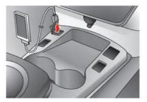
Connect the iPhone<sup>®</sup> cable to the USB connector. If the iPhone<sup>®</sup> supports charging via USB, the battery of the iPhone<sup>®</sup> will be charged while connected to the vehicle.
