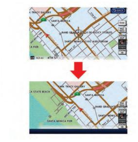
The basic map screen displays the current location (the position where the vehicle mark is located). Push the **MAP** button to display the current location on the map while on any screen.
