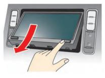
The angle of the monitor can be adjusted to select from 3 different preset angles. Once the angle of the monitor is selected and stored in the system, the selected angle is always set after performing the open/close operation of the monitor.
